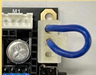
2.If you use 48V, you need to connect an external power supply to the 48-PIN and GND-PIN using the connecting wires provided by us.
